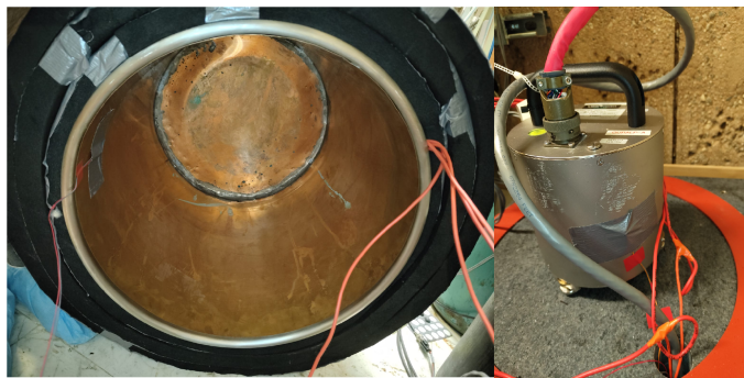
Figure 1: Seismometer setup. Left: the inside of the can, the foam is visible around the edge of the can; the red wires lead to the sensors and resistor used to measure the temperature and heat the can. Right: The seismometer device which rests inside the can.
