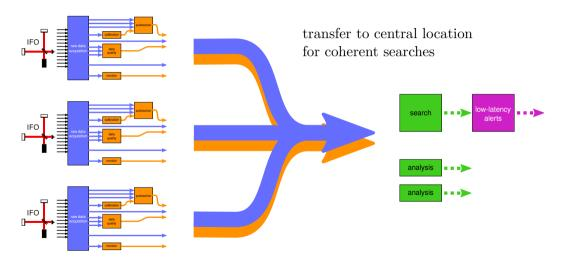
**stream processing**: Data Monitoring Tool (DMT) receives data from the DAQ in one-second long frames. Data passed between elements via shared memory. Applications must run in special environment, on a single machine.
