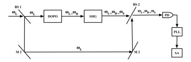
Figure 2: Homodyne detection scheme to measure the frequency noise of DOPO. The first arm is the one including DOPO and SHG, whereas the second arm is the one including AOM. The mirrors, M1 and M2, are highly reflective.
