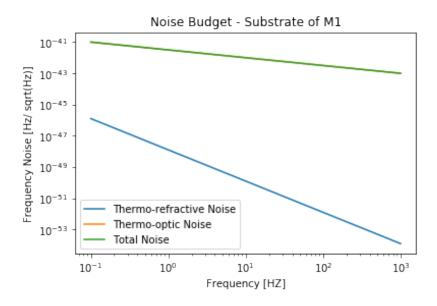
Figure 3: Noise Budget for the substrate of mirror 1. The noise introduced by mirror 2 will be identical to mirror 1.
