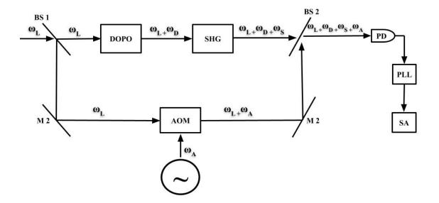
Figure 1: Heterodyne detection scheme to measure the frequency noise of DOPO. The first arm is the one including DOPO and SHG, whereas the second arm is the one including AOM. The mirrors, M1 and M2, are highly reflective. The angular frequency  $\omega_L$ ,  $\omega_D$ ,  $\omega_S$  and  $\omega_A$  represent laser frequency, DOPO's frequency, SHG's frequency, and AOM's frequency, respectively.
