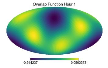
FIG. 4. The overlap function of H1 an L1 as a function of time at hour 1 of a sidereal day. The dark blue and yellow represent locations in the sky in which the detectors are most sensitive. As the sidereal day continues, the areas of high sensitivity rotate along with the detectors relative to a fixed point in the sky.
