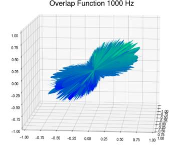
FIG. 7. 3D overlap function dependent on frequency at 1000 Hz. In this plot, the coloring aids in the 3D visualization and has no further significance. The axes represent the value of the overlap function at a given location.
