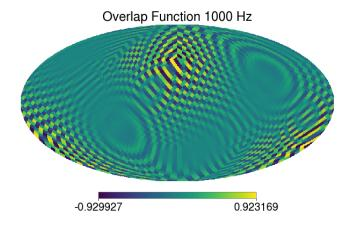
FIG. 5. The overlap function of H1 an L1 as a function of frequency at 1000 Hz. The dark blue and yellow represent locations in the sky in which the detectors are most sensitive. As the frequency increases, the number of waves that fit between the two detectors increases.
