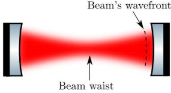
Figure 4: Laser beam front mode-matched with optical cavity
