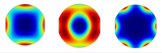
Strain energy density of different modes, clear that some modes have higher strain in the center or edge
