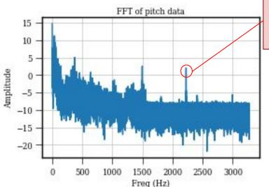
Eigenfrequency of excited mode: 2224.72 Hz
