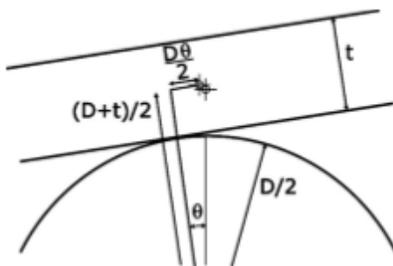
Figure 1: Diagram of Gentle Nodal Suspension system: the spherical structure touches the silicon disk at a single node. The silicon wafer is drawn as the angled piece suspended on the hemisphere.
