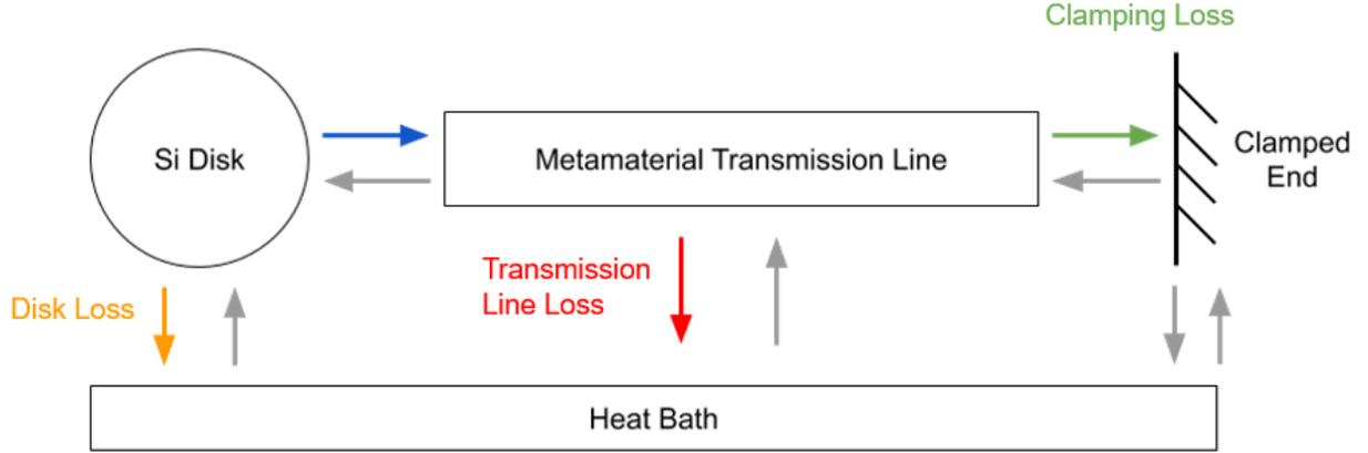
Figure 6: A schematic of the disk-metamaterial system. The energy propagating from the disk (blue) into the transmission line will result in mechanical losses (red) due to the stored strain energy. Any kinetic energy that escapes through the transmission line to the clamped end will be dampened, resulting in an additional clamping loss (green). We would like to design a system where these two additional loss terms are smaller than the disk loss (orange).
