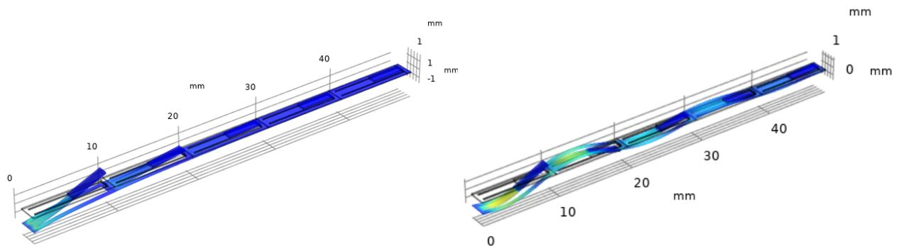
Figure 11: The transmission line response to transverse harmonic loads at 1kHz (left) and at 4kHz (right). The responses demonstrate different disk isolation mechanisms that the metamaterial can exhibit. The energy propagates further into the transmission line for the 4kHz case, which is less desirable from a mechanical loss standpoint.
