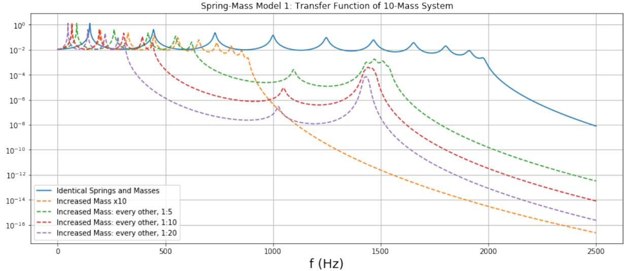
Figure 2: The transfer function for a spring-mass model where different resonators are connected in series. The blue curve is the case where all resonators are identical. For the orange curve, all masses are increased by a factor of 10. Bandgaps are present in the green, red, and purple curves, where every other mass (odd masses in Figure 1) was increased by a factor of 5, 10, and 20 respectively.
