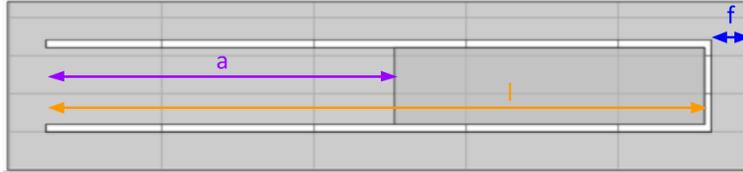
Figure 7: Top view of the cantilever geometry.  $a$  is the length of the thin part of the cantilever,  $l$  is the total length of the cantilever, and  $f$  is the frame width. These three parameters were the main focus of the optimization studies.
