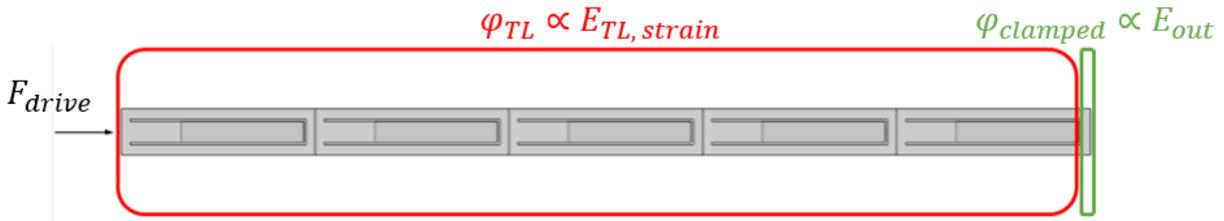
Figure 9: A top view of the transmission line model, divided into two regions where the strain energies can be measured separately. The strain energies from these two regions result are used to calculate the transmission loss and clamping loss of the system.
