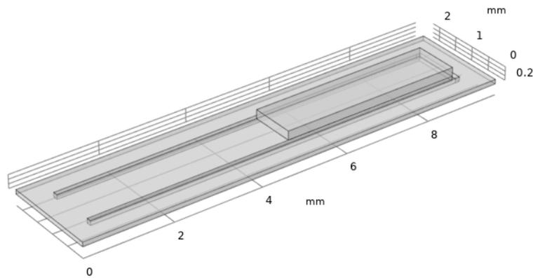
Figure 5: A model of the resonator unit cell constructed in COMSOL. The resonator consists of two components: a cantilever and a frame. The cantilever is attached to the frame on one end, and the other end has a thicker block to lower the resonance frequency. The frame is necessary to connect multiple resonators in series.
