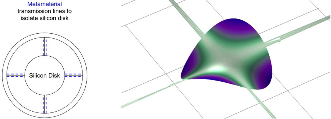
Figure 4: A schematic of the transmission line disk isolation system (left) and a visualization of the system behavior when the disk butterfly mode is excited (right). The system consists of four transmission lines patterned with resonators, connected to the disk at  $90^\circ$  spacings.
