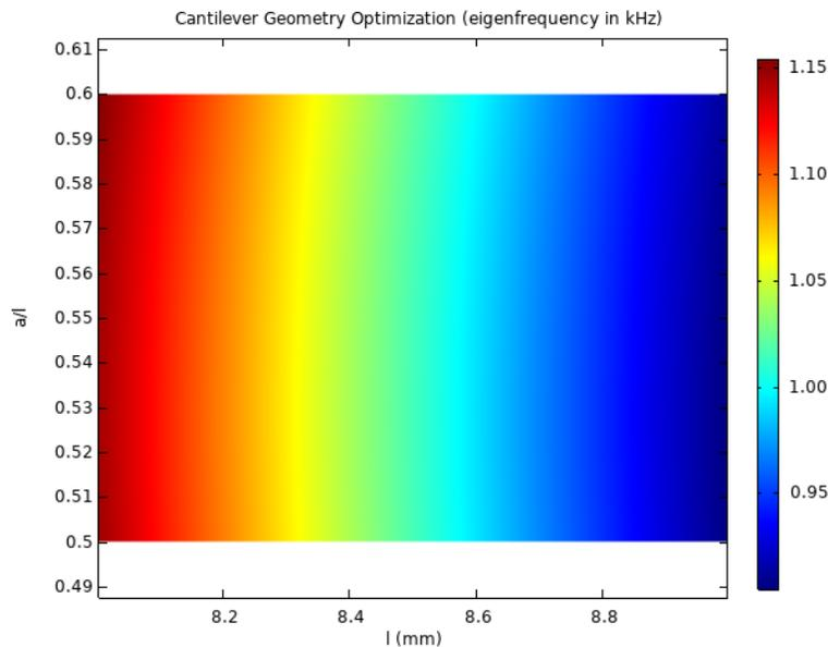
Figure 8: The results of a parameter sweep for the cantilever geometry, showing the eigenfrequency of the cantilever resonator as a function of the cantilever length and the fraction of the cantilever length that is thin. A 1kHz resonance can be achieved while maintaining a sub-cm scale resonator unit cell length.
