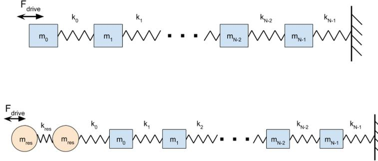
Figure 1: The top diagram is a spring-mass model in which resonators are connected in series. A driving force is applied to the mass on the left end. The corresponding transfer function is proportional to the displacement of the mass on the right end. The bottom diagram shows a high-Q resonator attached to the free end of this configuration. The resonator is comprised of two masses and a spring, with a resonance frequency reflecting the value for the silicon disk mode.
