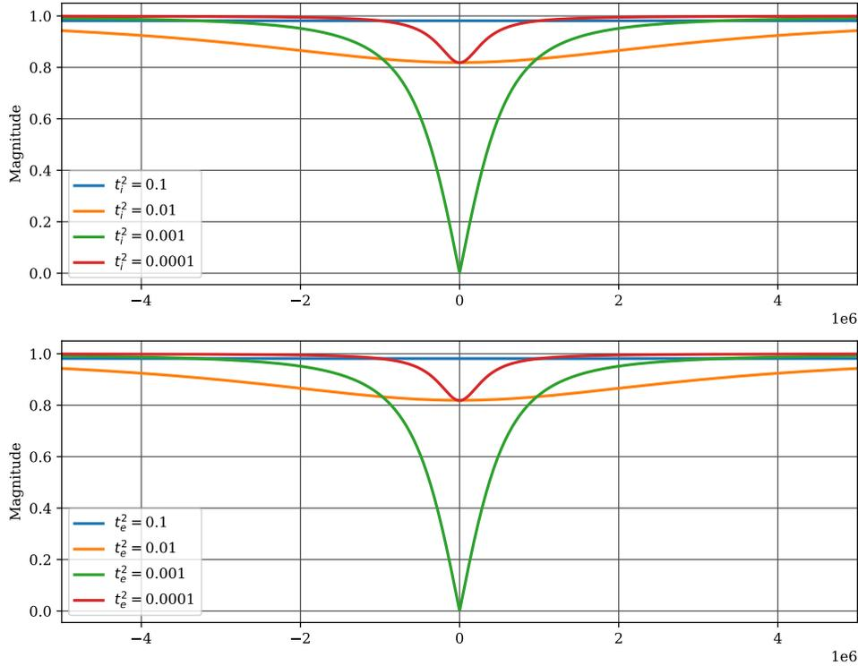
Figure 1: The first plot holds the input mirror transmissivity at 0.1% and modifies the end mirror's transmissivity and shows the results for values of 10%, 1%, 0.1%, and 0.01%. The second plot does the reverse, and holds the end mirror transmissivity at 0.1% and modifies the input mirror for the same values. The plots are identical due to cavity losses being ignored.
