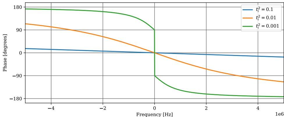
Figure 2: This is a plot showing the phase of the Fabry-Perot cavity as a function of the frequency, where  $t_e = 0.001$ . When  $t_i = t_e$  for the green curve, there is a 180 degree phase change, indicating that the cavity is critically coupled. The other curves are undercoupled, i.e.  $t_i > t_e$ .
