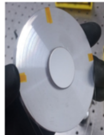
Thermal Deformable Mirror (CIT/Adelaide)
