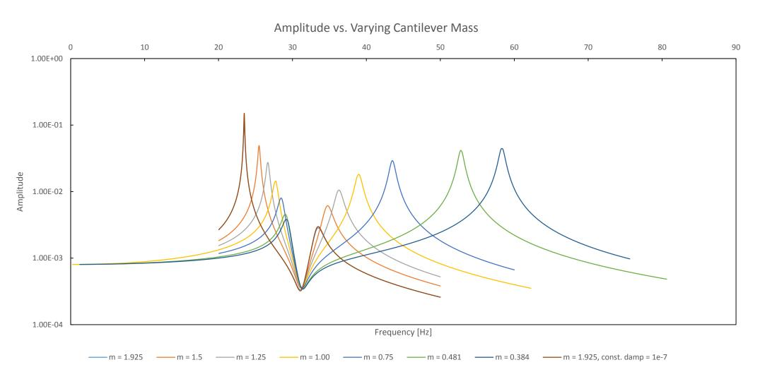
Damper frequency  $f_d = 31.19$  Hz. Low peaks (20-30 Hz) correspond to cantilever frequency; high peaks to damper frequency. Lines correspond to varying mass of cantilever (in kg).
