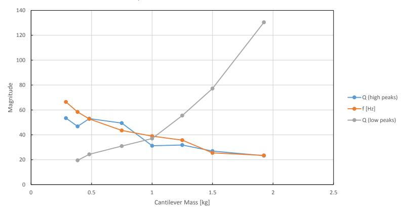
• Original cantilever mass  $m_0=0.384~{\rm kg}$  and mass of damper  $m_d=0.06~kg$ ; simulation ranged from  $0.75*m_0$  to  $30*m_0$ . Resonant frequency of damper  $f_d=31.19~{\rm Hz}$ .
