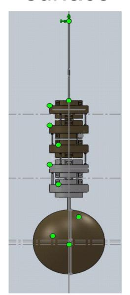
System composed of the copper cable with a diameter of 0.5 mm and a radius of 80 mm connected to a cylindrical mass, called a rigid mass. The rigid mass on the right is used in the model to take into account the effect of the sphere suspension on the cabling. The excitation considered acts on the left end of the cable.
