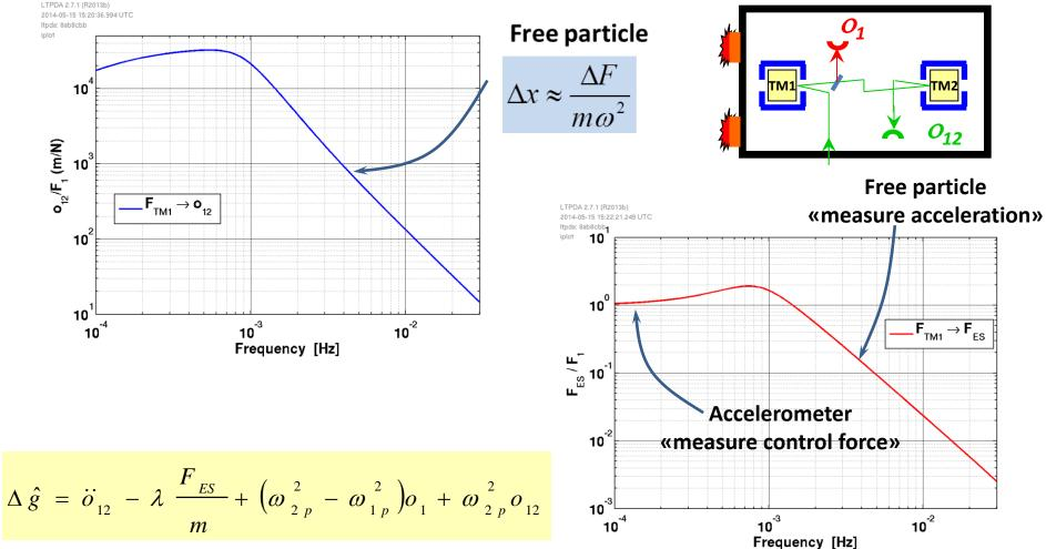
Need to calibrate actuator and SC coupling (stiffness)
