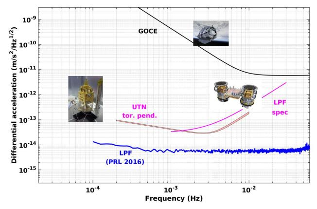
Pre-flight torsion pendulum tests retired some GRS force risks
