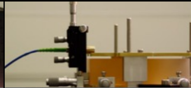
template aligned to beam
