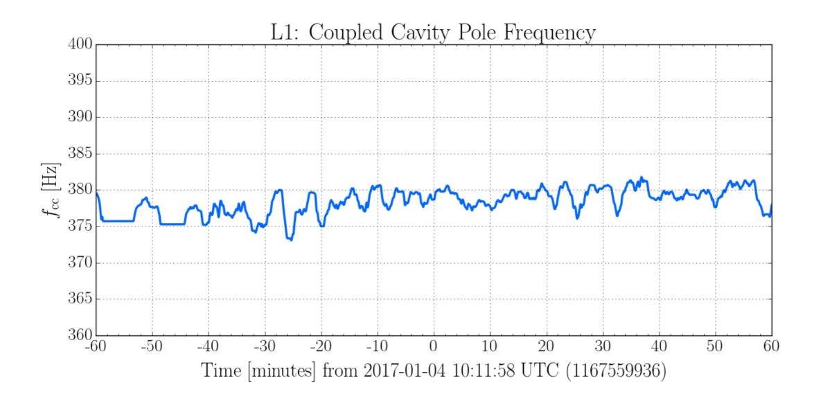
however, the coupled cavity pole is a time-changing corner frequency in a low-pass filter (the sensing function)
