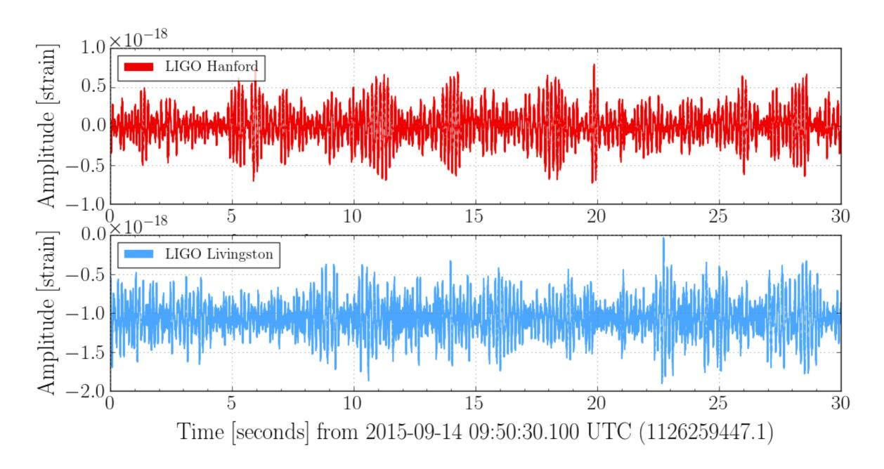
raw timeseries output can have DC offset, must be bandpassed (and notched) to visualize signals
