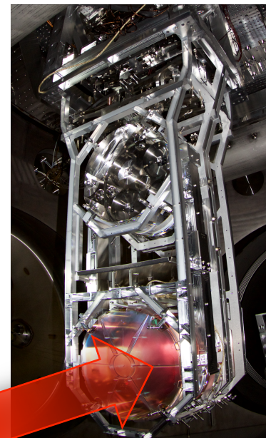
Fabry-Perot cavities in the Michelson arms ~100kW laser power in O1
