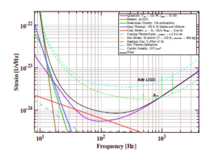
Low temperature (123 K) operation of the 150 kg Silicon test masses
