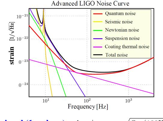
**100Hz signal (1sec long):**  $h_{\min}|_{100\text{Hz}} \approx \sqrt{S_{nn}(100\text{Hz})\Delta f}$  $\Delta f = 1/\Delta t = 1\text{Hz}$   $\approx 10^{-23}$
