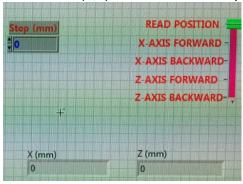
9. The down direction is the Z positive axis and the left direction is the X positive axis. To calibrate with the 3:00 position, enter 20mm into the "Step" box and move the slider to "Z-axis forward." Click the run button. Note: you are really moving 10mm due to the software.
