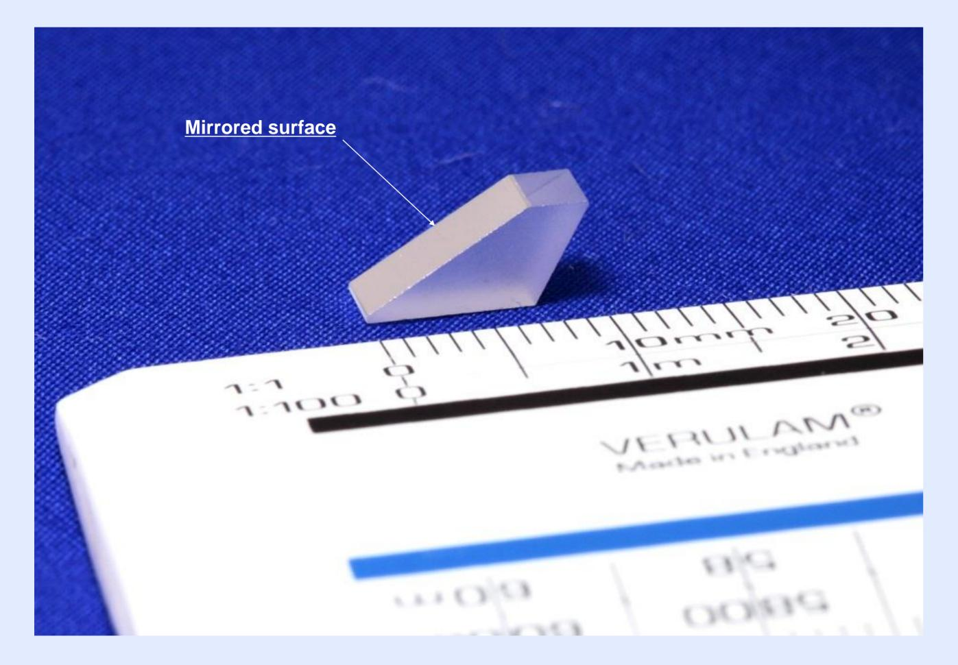
The displacement-doubling prism [1]. Its entrance- and exit- windows whose designation is interchangeable—are plane-parallel, and light enters and exits these at normal incidence, so that the prism is nondispersive. When the prism is displaced laterally relative to an incident light beam by an amount  $\Delta x$ , say, then the exit beam will be displaced laterally by  $2\Delta x$ .
