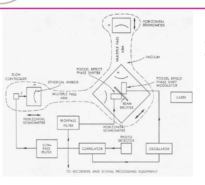
Not first suggestion of a laser interferometer to measure GWs, but first detailed noise/ sensitivity analysis
