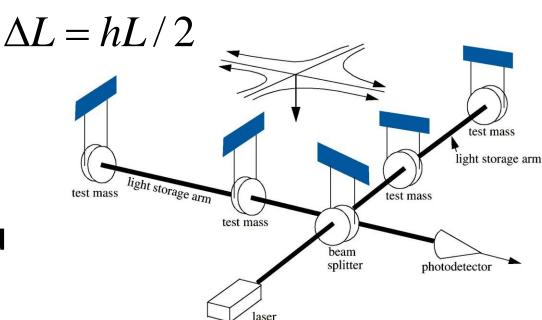
For a LIGO L = 4 km For  $h \sim 10^{-22} - 10^{-21}$ ,  $\Delta L \sim 10^{-18}$  m (~1/1000 diameter of proton)
