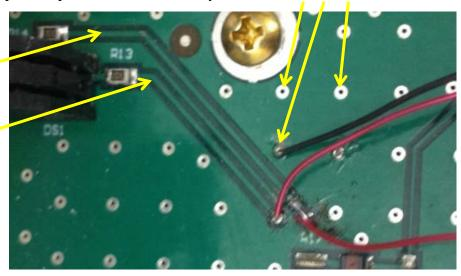
These three places have vias into which a wire-wrap wire can be inserted and soldered. The Status 2 via in the picture above was slightly lifted, so I soldered it to the trace, instead. These wires are then inserted into the connector thusly:
