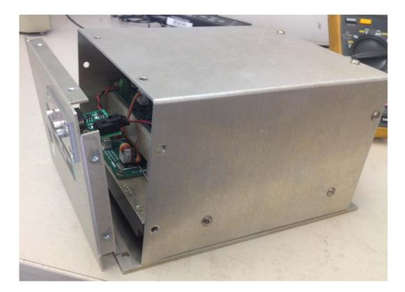
Now, plug in the connector, and attach the back panel with the six roundhead screws and 2 countersunk screws. At this point the modulator should be powered up with +24V and GND, and a separate 5V-to-GND should be supplied to pins 1(+) and 7(GND) of a 9-pin breakout attached to the AOM Mon connector. With no AOM plugged in, both LEDs should be red, and pins 6 and 2 should read +4.3V to pin7 (GND).
