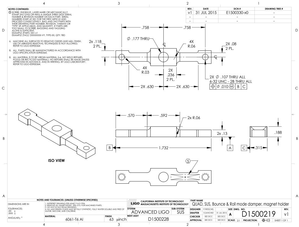
D1500219 QUAD, SUS, Bounce & Roll mode damper, magnet holder, PART PDM REV: X-000, DRAWING PDM REV: X-000
