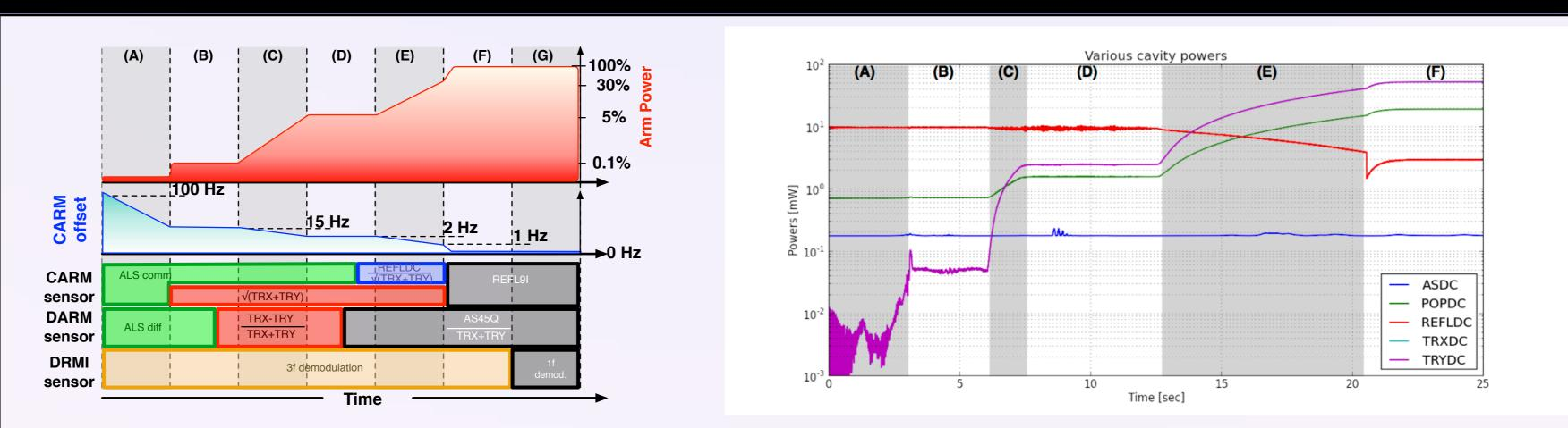
We introduced an offset in CARM for locking DRMI. Then the offset was reduced while the sensors for DARM and CARM were sequentially switched in order to have higher signal-to-noise ratio.
