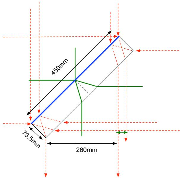
**Figure 3 BS geometry and clear aperture**
