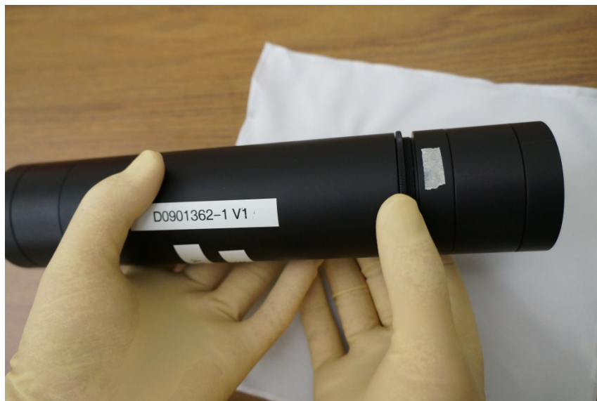
Fig. 4 Adjustment of the objective gap. The adjustment of the objective gap is straight forward by releasing the lock ring which holds the 2” objective mount tube fixed, then turning it (0.635 mm/turn).
