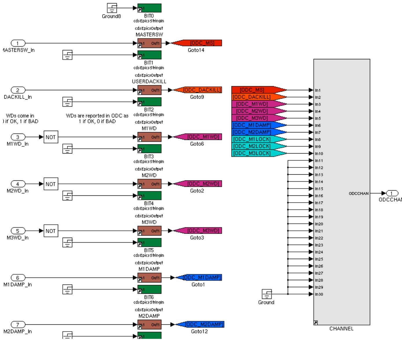
All bits get piped into new ODC V2 Block which is much cleaner
