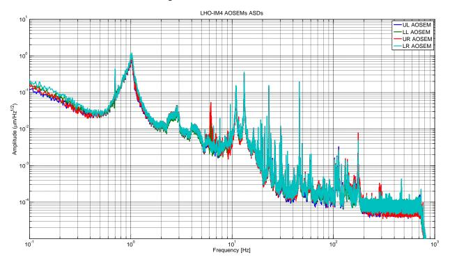
There are no requirements associated with this measurement. It is rather intended to be a sanity check looking for strange behaviors and differences between OSEMs. As a reference, high frequency electronic noise is expect to be  $\sim 10^{-4} \, \mu m/Hz^{1/2}$ .
