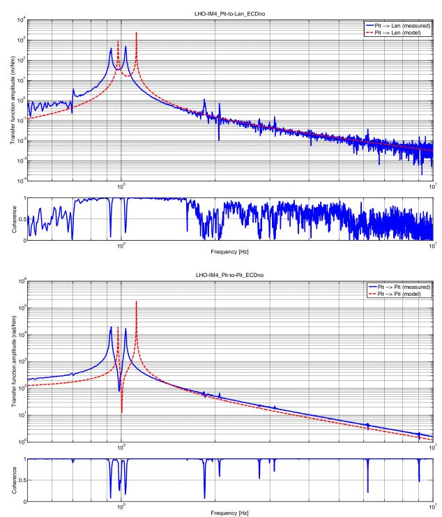
Possible double peak visible at the lowest resonance. However, the coherence in that region is low and there is no other indication of anomalies in the remaining TFs.
