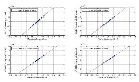
There are no requirements associated with this measurement. It is rather intended to be a sanity check looking for strange (e.g. non linear) behaviors and differences between OSEMs. <u>Passed</u>
