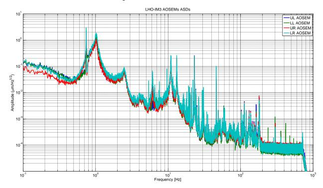
There are no requirements associated with this measurement. It is rather intended to be a sanity check looking for strange behaviors and differences between OSEMs. As a reference, high frequency electronic noise is expect to be  $\sim 10^{-4} \, \mu \text{m/Hz}^{1/2}$ .
