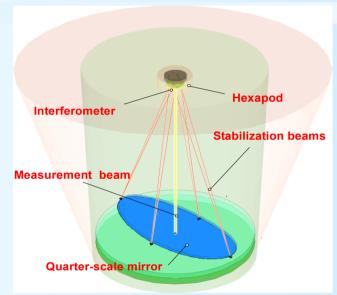
Measurement of primary mirror thermal stability to  $10^{-10}$  m over 8 hour: "Stabilized Metrology"
