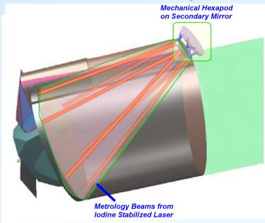
Stabilized laser and hexapod control of secondary mirror to 10-8 m over 8 hour
