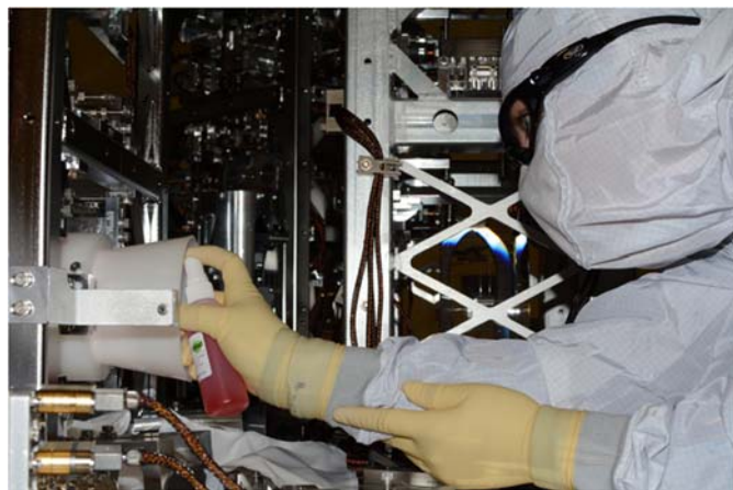
Figure 10. Person 2 spraying FC onto PRM with nozzle at the max acceptable distance from the optic face
