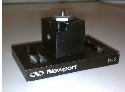
Figure 1: Triple-axis accelerometer mount used in iLIGO.
