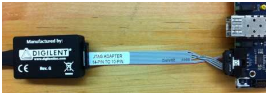
Top view of adapter: 14-pin side of adapter, left, connected to XUP USB-JTAG Adapter
