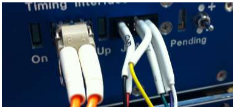
10-pin JTAG port with flying wire adapter connected
