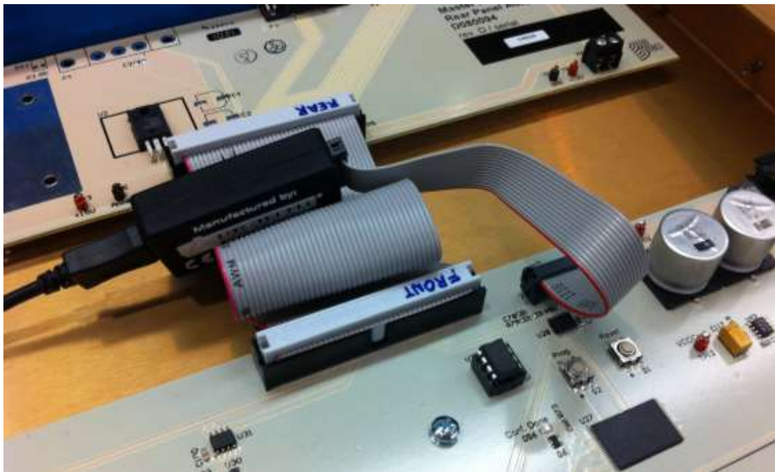
Timing Master connected via 14-pin to XUP; view from front of chassis
