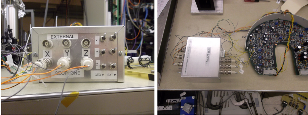
Figure 19: The signal box which allows for feedforward and/or feedback isolation. In the picture to the right it is connected to the preamplifier; everything is plugged in as usual to the STACIS, except several BNC cables are connected to the box when it is being used. Similarly, BNC cables connect to the external signal (from seismometers, in a feedforward isolation scheme).
