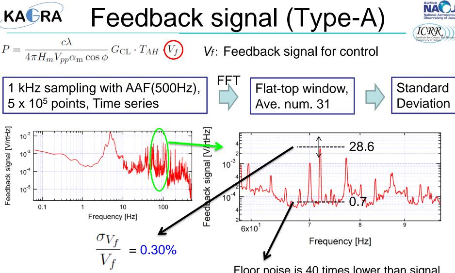
★Including Intensity noise, thermal drift and so on. Floor noise is 40 times lower than signal  $(1/40)^2 = 0.000625 \approx 0.06\%$
