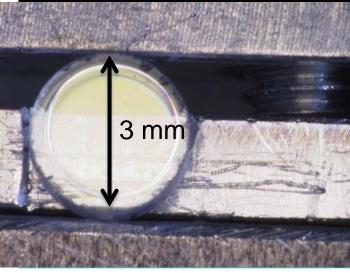
Beam spot size: w = 0.2 mm  $\Rightarrow w \ge 0.4 \text{ mm}$  area include 99.97% of power
