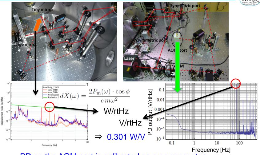
PD on the AOM port is calibrated as a power meter
