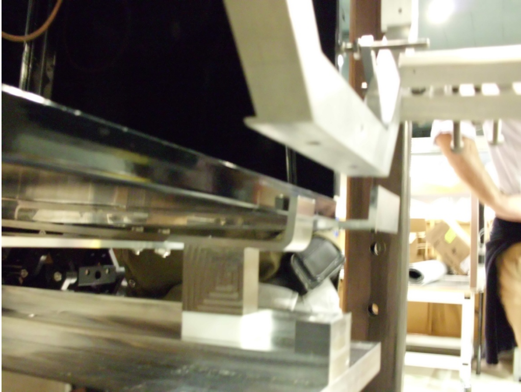
6.3.10 Pull Slide Assembly along Rail Assembly to end toward spool, and leave it there until later removing through the manifold tube.
