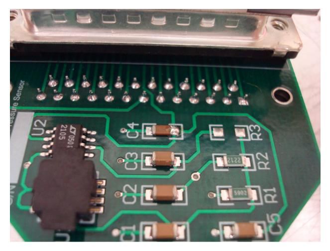
Here's the TVS in place hunkering over C4 with both sides soldered:
