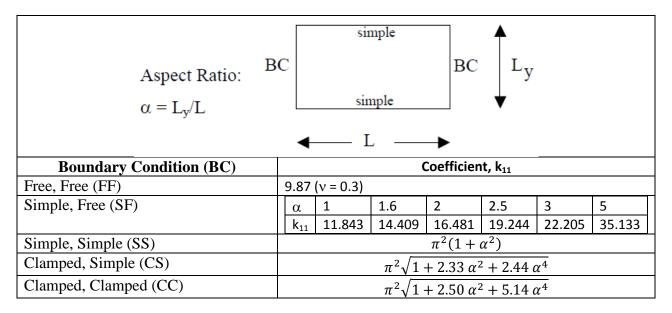
The panels of the PCal pylon can be roughly approximated by rectangular panels which have simple supports on 3 sides and 1 free edge with L = 0.24 m, Ly = 0.36 m,  $\alpha$  = 1.5, as shown in the Figure below.
