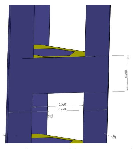
With simple-free boundary conditions (BC) then  $k_{11}$  = 14.1, D = 120 Pa and f = 49 Hz.
