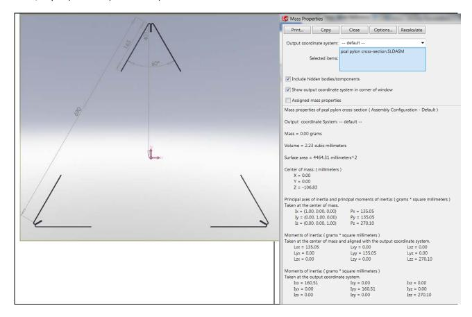
To determine the area moment of inertia, divide the solidworks moments of inertia by the density and the depth (i.e. divide by  $10^{-6}$ , and then convert to m<sup>4</sup> (from mm<sup>4</sup>; divide by  $10^{12}$ ), so I = 1.35 x  $10^{-4}$  m<sup>4</sup>
