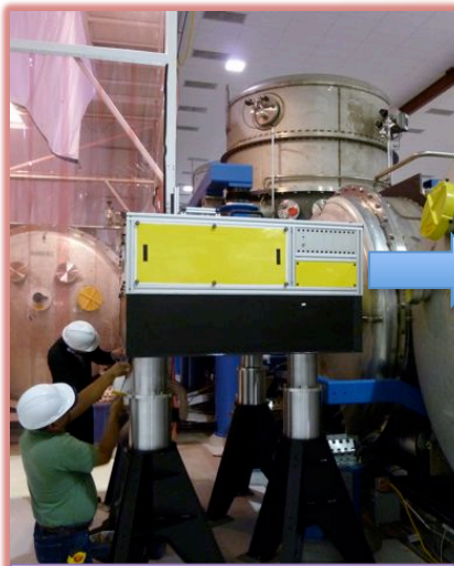
Squeezer table craned to its final location
