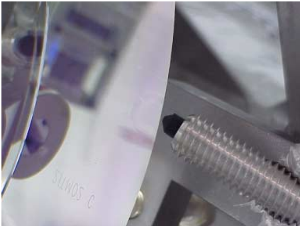
FIGURE 2. Close-up photograph of the new conical tip and the small spacing (0.5 mm) to the edge of the suspended optic to limit motion.
