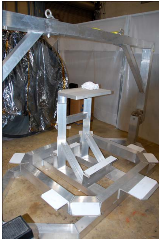
Figure 1: Manifold/Cryopump Baffle Lift/Assembly Fixture
