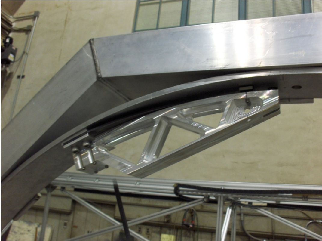
Figure 20: Top Suspension Ring Mounted to Alignment/Balance Fixture
