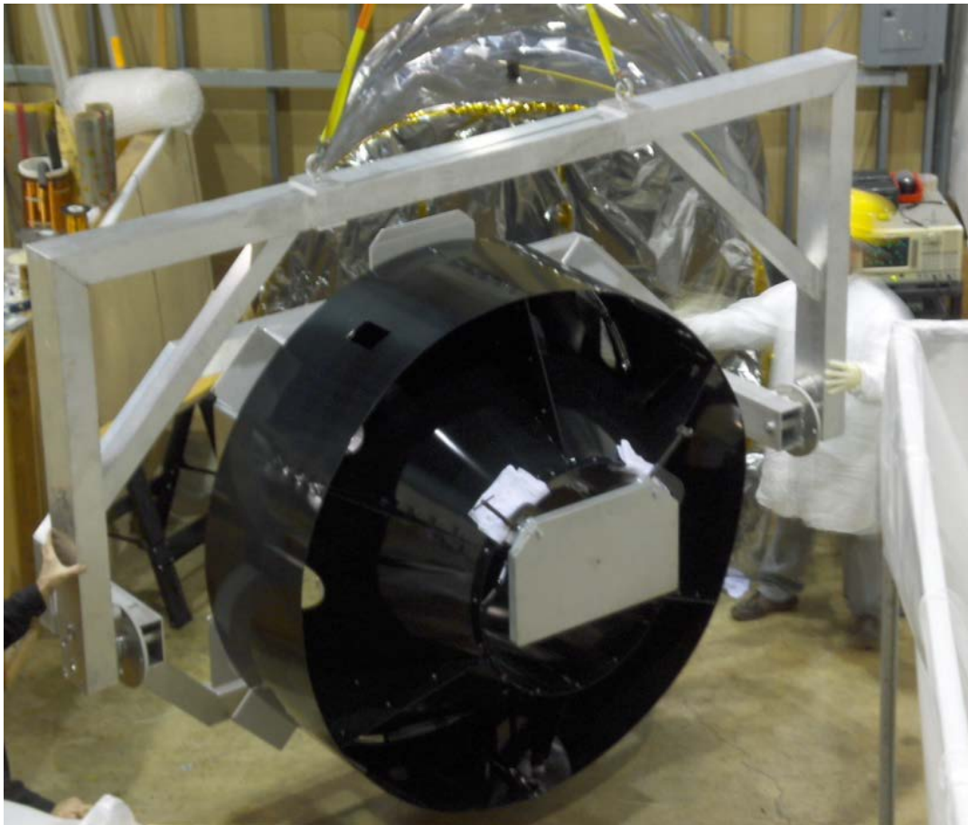
Figure 23: Lift/Assembly with Baffle Supported by Crane
