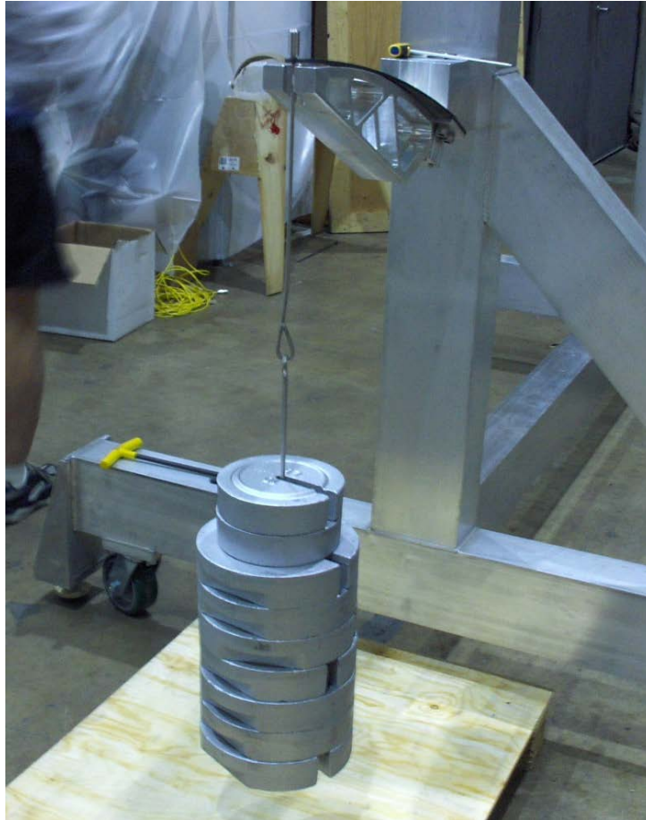
Figure 18: Pre Load Spring Blade by Hanging Weights
