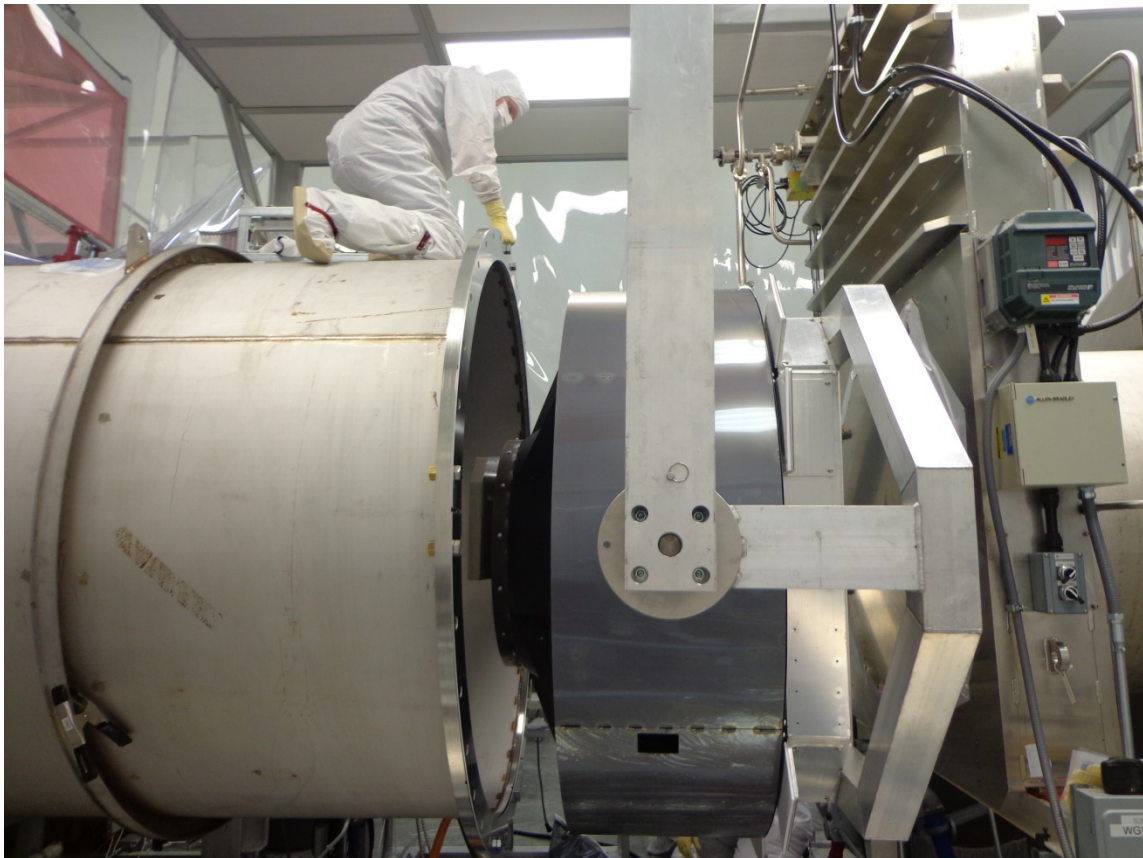
Figure 34: Baffle between spool and gate valve
