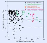
Figure 7: The breaking stress of fibres heated for alignment a few mm outside of their neck or not heated at all. Fibres pulled using the H2-O2 flame and CO2 laser are
