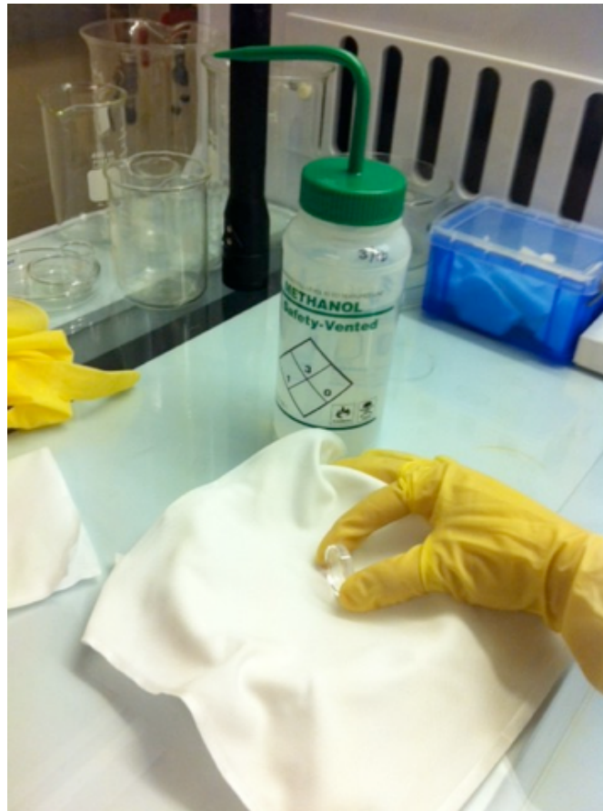
Figure 1: Example of how to hold a 1" optic, in the cloth covered petric dish.
