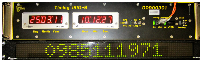
IRIG-B Timing Fanout Provides accurate time information to computers.
