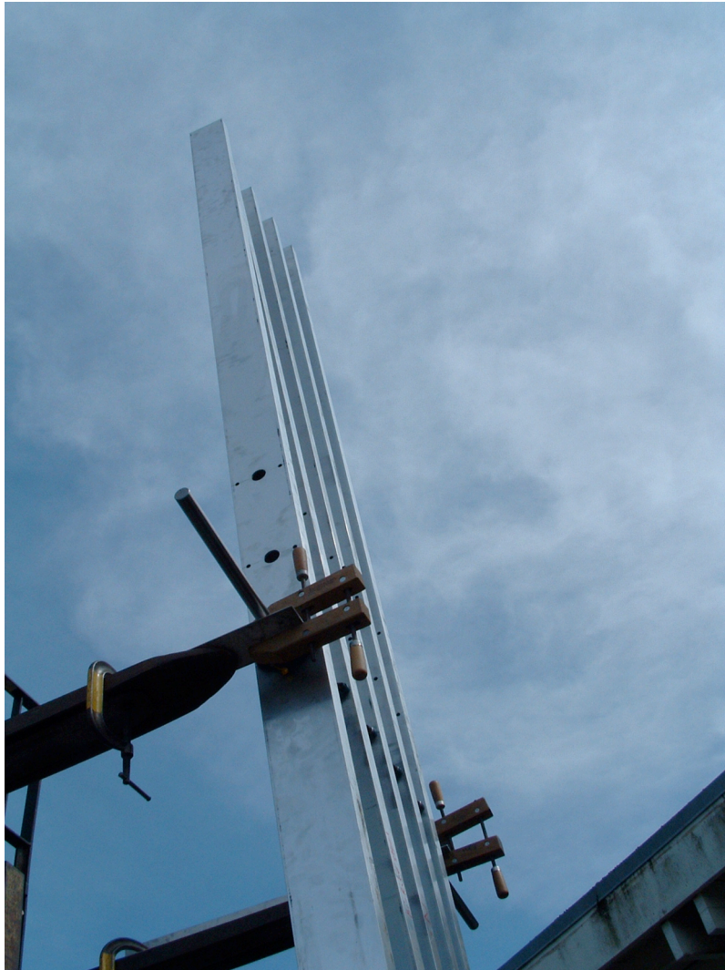
Figure 2: Test of a short section of magnetically coupled kinetic pendulum façade at the Exploratorium in March 2005. (M. Zucker, LLO)
