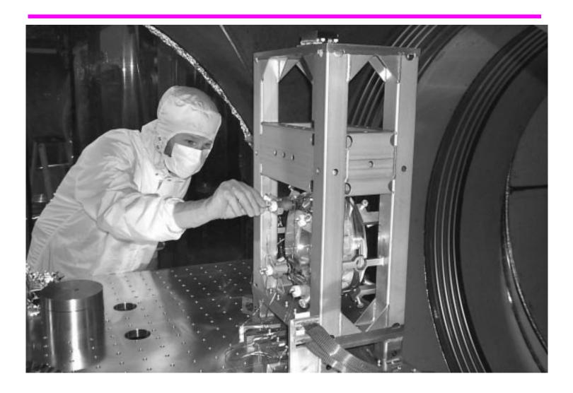
Combination of 5 major subsystems (Core Optics, Suspension, Seismic Isolation, Initial alignment, CDS)
