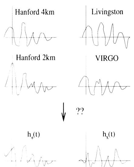
• Such algorithm useful for (i) obtaining GW waveforms after detecting signal, and (ii) Constructing a multi-detector veto (subtract from all detectors best fit signal).
