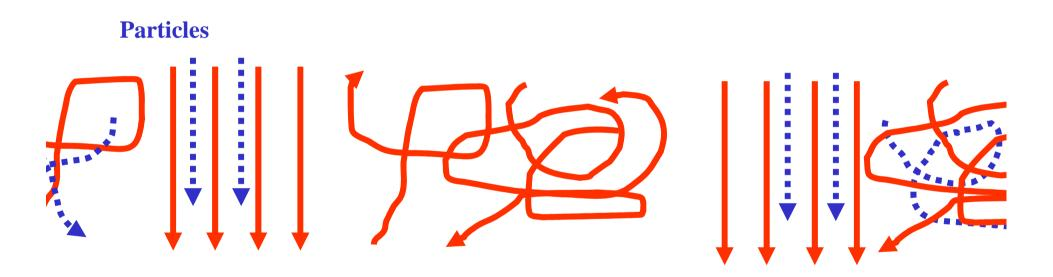
The particles, are dragged away by the flow before they can diffuse in the turbulent flow volume. But high turbulence induced in the optics region can still generate particulate contamination Diminished but not negligible polluting probability
