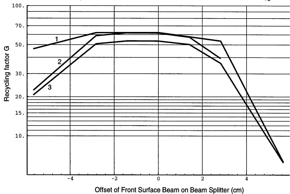
Calflat mirror surface maps and 50 ppm base loss per mirror surface. Curve 2 and 3 are for  $\phi_s = 25 \text{ cm}$ ,  $d_s = 4 \text{ cm}$ . Curve 2 employs the same mirrors as Curve 1.
