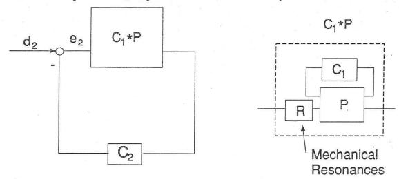
Better sensing scheme will not reduce  $S_{22}$  (assuming  $C_1 \ast P$  is well-behaved within the bandwidth of the  $C_2$  loop).  $S_{21}$  can be reduced by using a better conditioned sensing scheme. This will improve performance if
