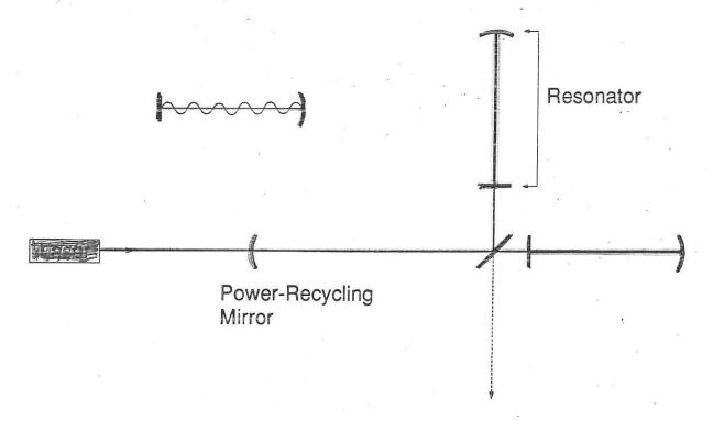
Recall: all mirrors are suspended from wires; swing around because of seismic ground motion (typically  $4 \times 10^{-7} \text{ m}_{rms}$ ).
